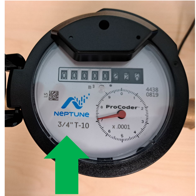
3/4 inch water meter
